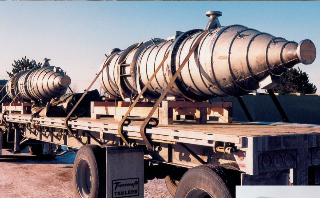
Stainless steel reactor vessels built to rigid customer specifications and tolerances.
