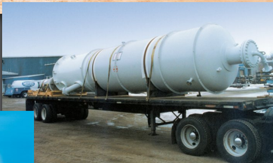
▲ FCC Stabilizer tower for the petroleum industry. 12' diameter x 125' long, weighing 140 tons.
