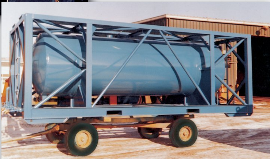
A transportation storage vessel complying with DOT specifications, ISO, and ASME codes is prepared for shipment.
