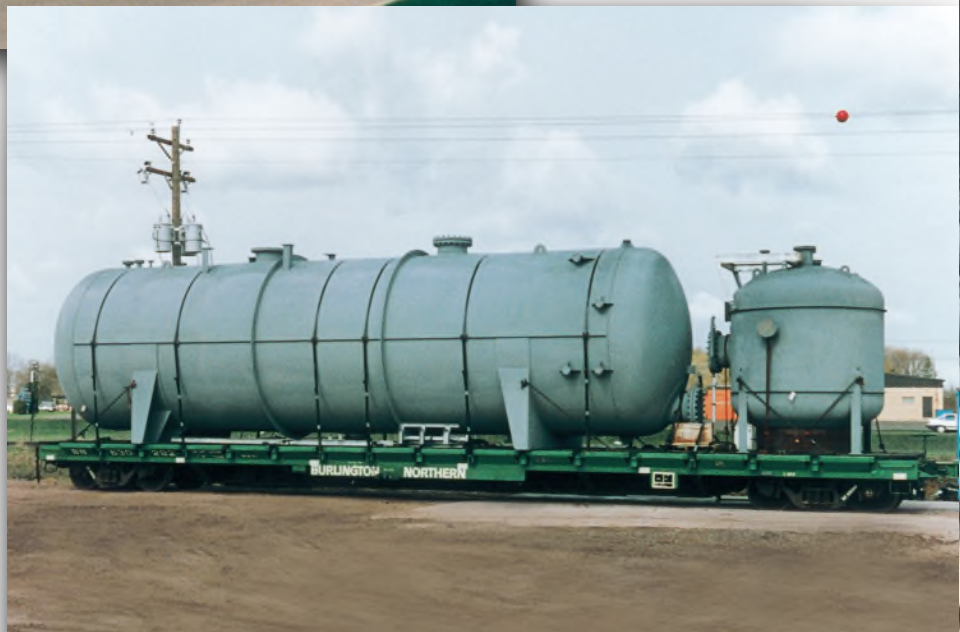
Completed deaeration unit for rail shipment to the Port of Houston, Texas. ►
