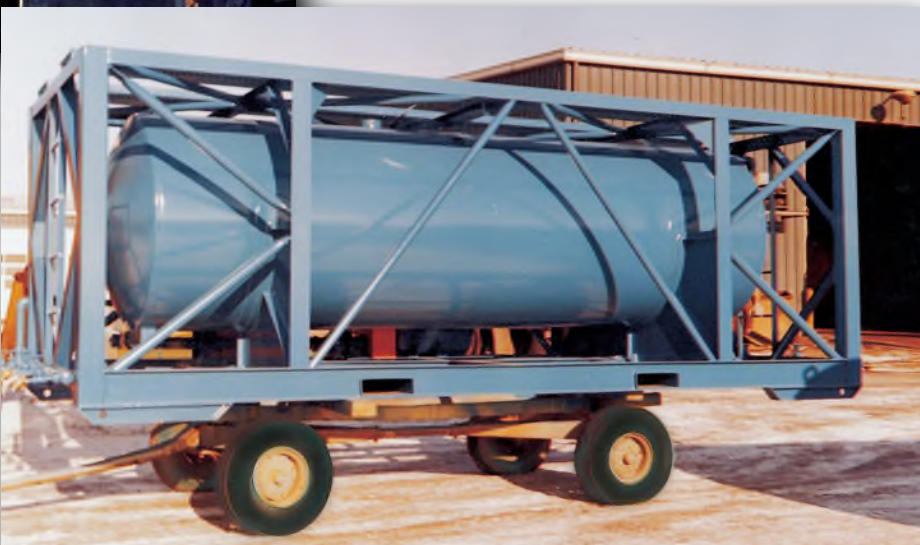
A transportation storage vessel ▶ complying with DOT specifications, ISO, and ASME codes is prepared for shipment.
